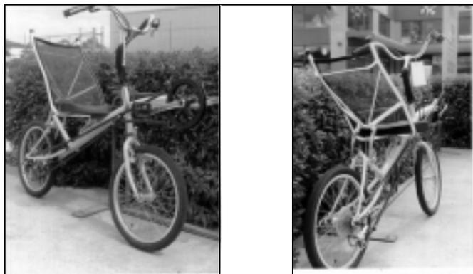
*Front and rear photographs of the Wavey recumbent showing the composite seat and general detail.*
