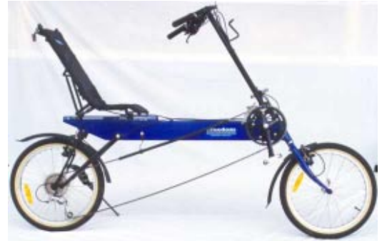
Breeze, a compact long wheelbase recumbent bike.
