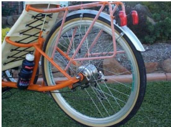
It is a stable and solid unit, yet responsive. Positive steering but light enough to be two-finger control when under way. Take the hands completely from the steering posts and the track is true. Yes, like any trike, sharp cornering can lift a wheel. With a little care, this isn't an issue and after a 5-minute learning curve I felt completely at home on it.
