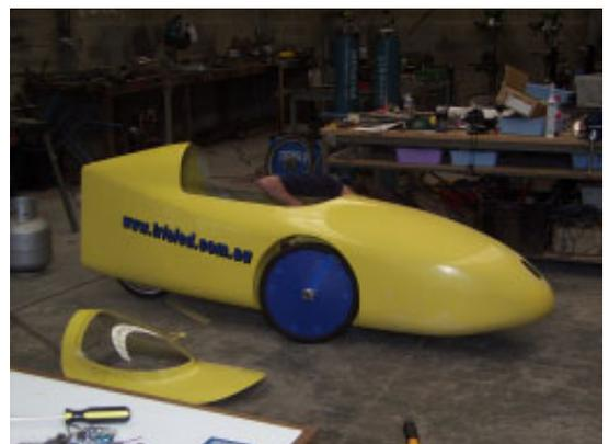
The first new fairing and frame to be fitted inside. Frame is structurally similar to our new Gizmo model although some
