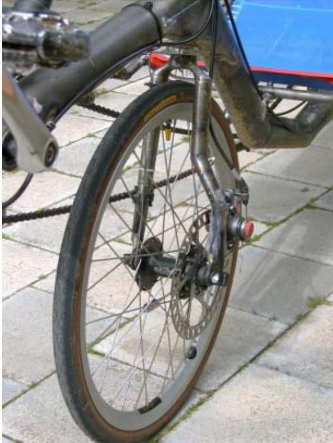
only one smallish gusset around the head tube junction this time. The other two joins have internal diaphragms in the junction of the tubes to resist bending and ovalising. The diaphragms are discs of 0.9mm sheet which are incorporated into the TIG weld of the two tubes. The boom tube is made from a length of the 50mm cro-mo, trimmed lengthwise with an angle grinder and reduced in diameter to 47.6mm approx with several hose clamps, then TIG welded along the join.
