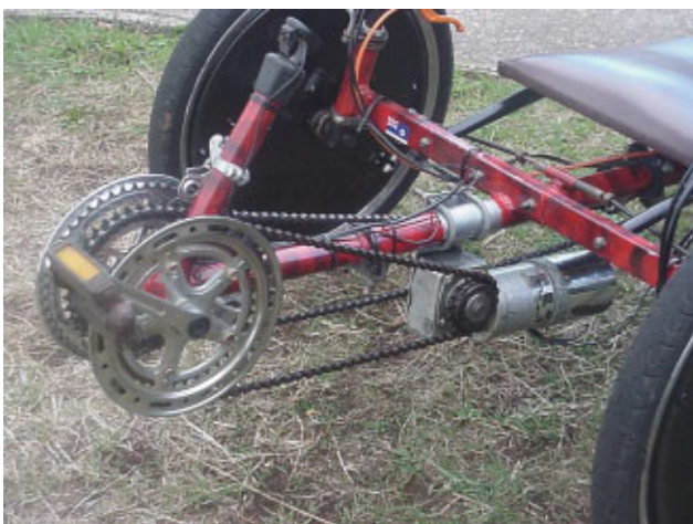
Robin 2 stroke engine driving a pancake generator. An electric motor drives the cranks from small gel batteries charged by this unit.
