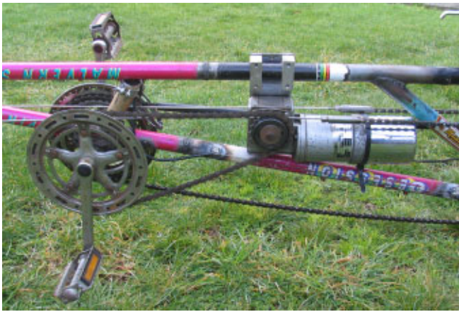
Ex electric wheel chair motor driving the cranks.
