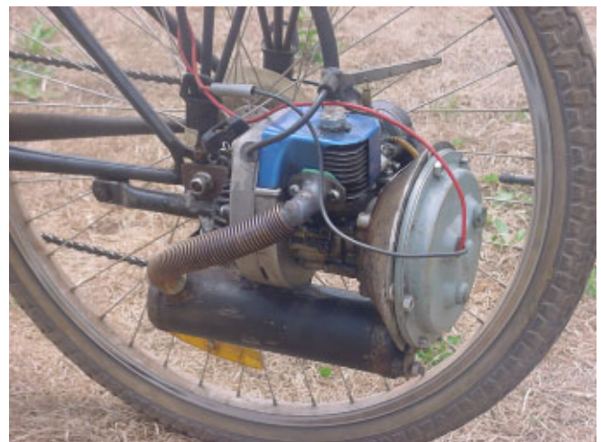
Robin 2 stroke engine driving a pancake generator. An electric motor drives the cranks from small gel batteries charged by this unit.
