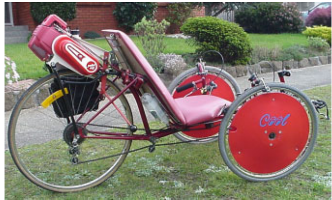
The rubber roller is geared down by a toothed rubber belt.
