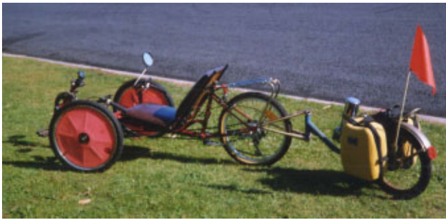
Ex electric wheel chair motor on a detachable trailer.
