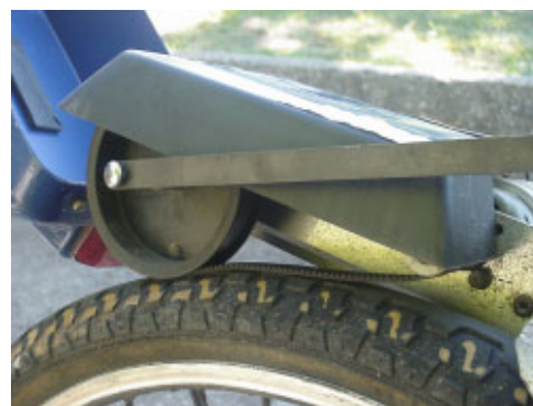
Zeta roller +belt on the tyre electric unit. Belt wraps around the tyre producing less slippage and wear.
