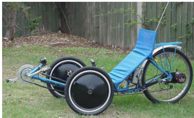
US Pro drive 24 volt kit - battery incl fuse and switch under the seat.
