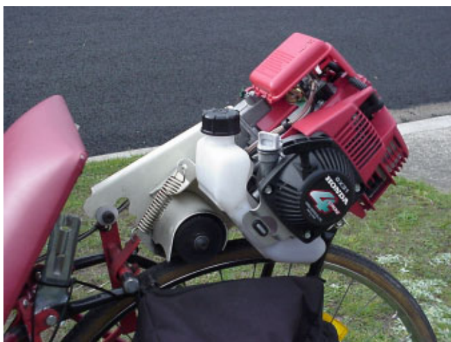
A Pedal Ezy with 4 stroke Honda 'roller on the tyre' unit.
