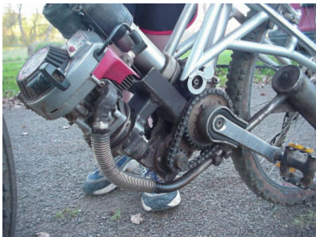
Robin 2 stroke engine connected to the pedals through a 50:1 gearbox. Rider has to pedal when the motor is driving the cranks.
