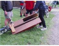
supposed to be a collapsible bike. Two Boxy bikes could be joined up into a tandem. The frame was two empty plywood boxes with front and rear mechanical subframes. The mechanical parts were meant to pack into the boxes to form a big suitcase. In practice, the boxes were really huge and I still couldn't get all the bits inside.
