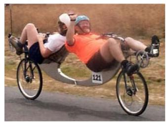
rivetted aluminium sheet construction, independent drives with a reversing chain for the back wheel and a twisting chain for the front, cranks with reversed threads, lots of rivets and a beguiling art-nouveau shape. Flevo founder and engineering genius Johan Vrielink was firing on all cylinders when he concocted this thing.
