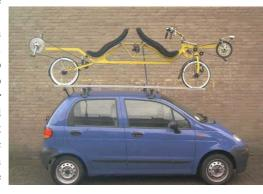
That bike has two structures running forward from the front of the seat – one is the fixed boom carrying the Bottom Bracket ('BB'), and below that is a suspended swingarm, carrying the
