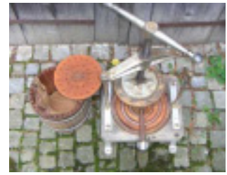
[Figure 5] Overview of press components. Note the cloth bag.
