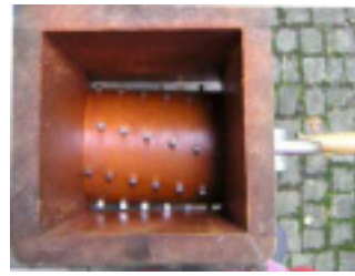
[Figure 4] Detail of the pulper's cylindrical rasp.
