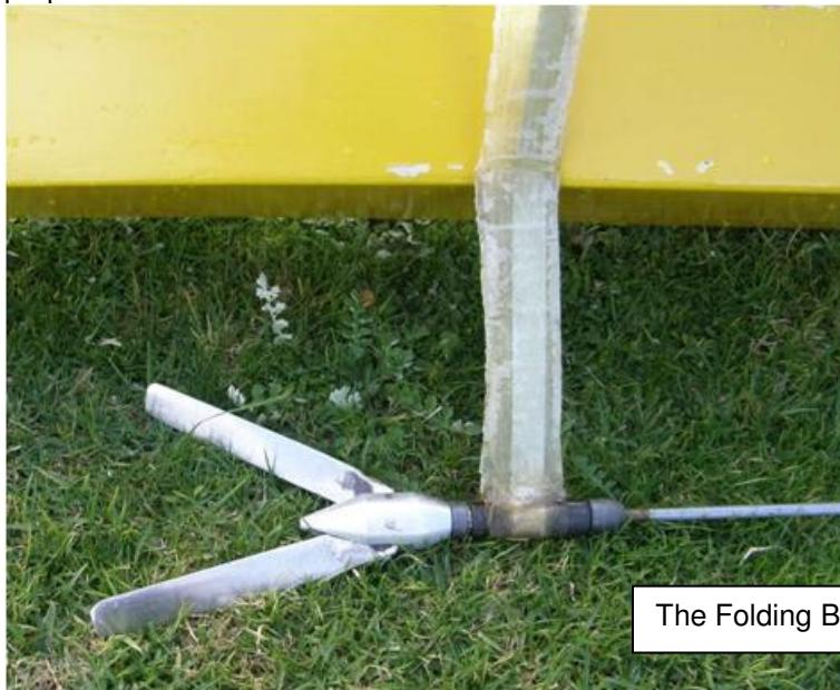
Rick is now working on V15 (yes that's version 15) of his pedal powered boats and says his sister wants a boat like his so he is working on an integrated hull design for her with a target weight of 15kg. It's Pink too. Note there is no chain – just a direct drive gear box to the propeller shaft.
