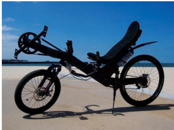
I have been building my own bicycles for the last 15 years and my latest creation, my third recumbent, incorporates a drop handlebar (road bike handlebar). With all my recumbents I have always used the Rohloff SpeedHub. Among its many attributes, the Rohloff hub allows gear changing whilst stationary, a most desirable feature on all recumbents.
