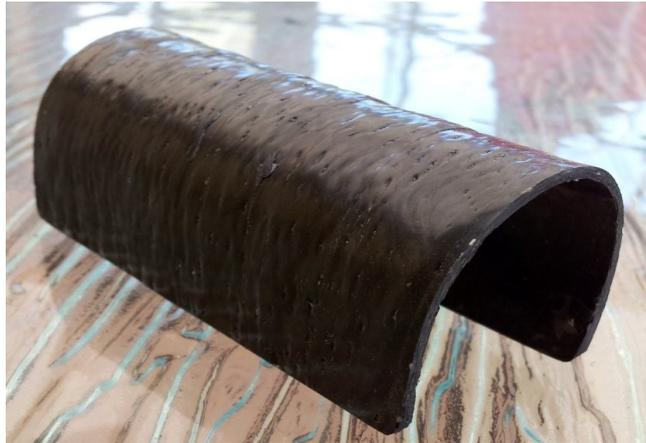
**Formed Damper: The electric tape compression leaves undulations on the surface**
