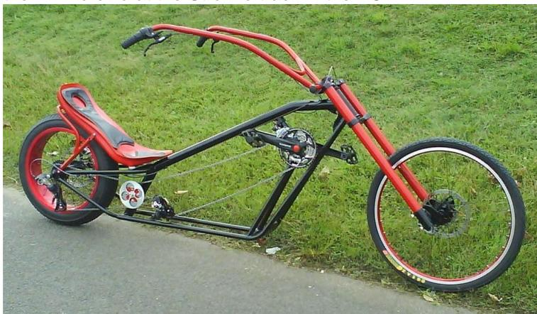
It did look the part but wasn't quite what I'd intended, more the later, racing model. Bit too low, bit too short for me, and of course being a prototype it was heavy. That middle stepout cog kept derailing, the front shifter never worked properly, and you had to remove the calliper to get the front wheel off. Worst of all, the forks rake/trail geometry hadn't been considered so the forks tended to flop to the side and the steering felt twitchy.
