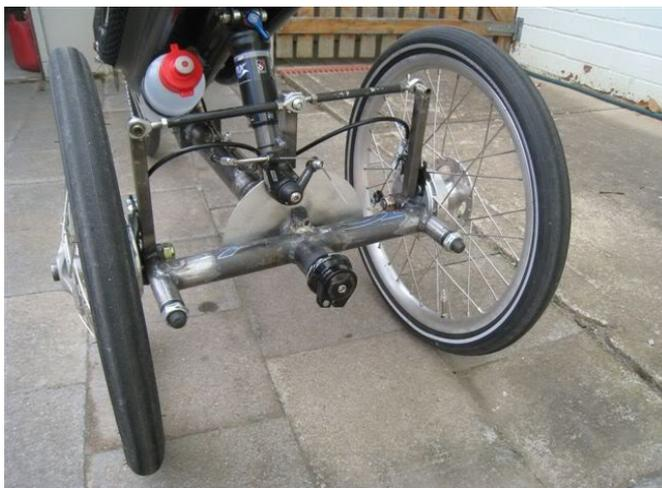
**Steering Lockout Mechanism**
