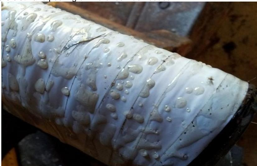
With all the cloth and Kevlar in place on the former, smooth the layup to remove air and wrinkles, then remove your gloves and put on fresh ones. Wrap electrical tape, sticky side out moderately tightly over the layup, piercing it as you go.
