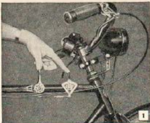
Sprocket ratio is selected by dual control levers which operate cables leading to shifts on rear wheel
