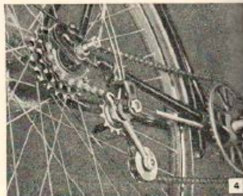
Below, shifting sprocket, operated by cable, travels sideways to throw chain from one sprocket to another. The idler takes up slack in chain when shifting
