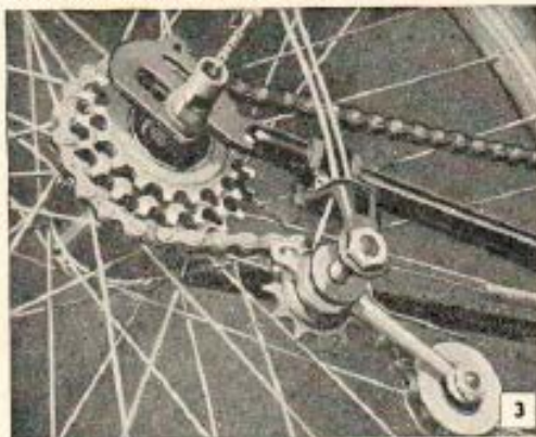
Below, close-up view identifying component parts of mechanism. The shifting sprocket and takeup idler which are integral clamp directly to bicycle frame
