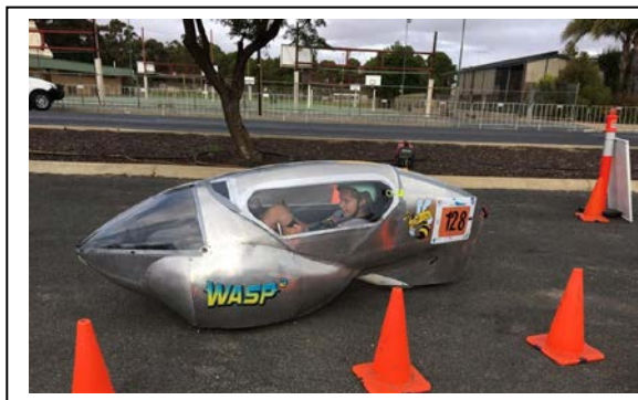
Yahl Primary's Aluminium monocoque, PACII mileage marathon car.
