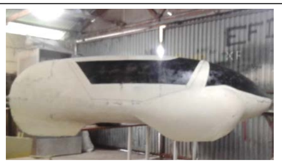
Plug used as shell mould, Composite velomobile nearing completion
