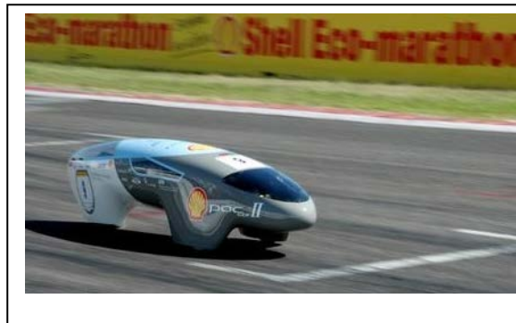
Yahl Primary's Aluminium monocoque, PACII mileage marathon car.
