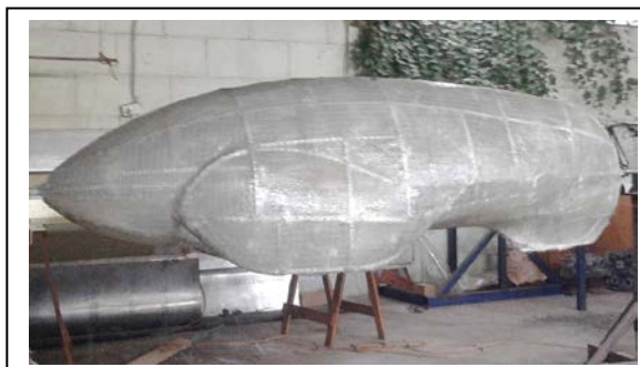
Plug used as shell mould, Composite velomobile nearing completion
